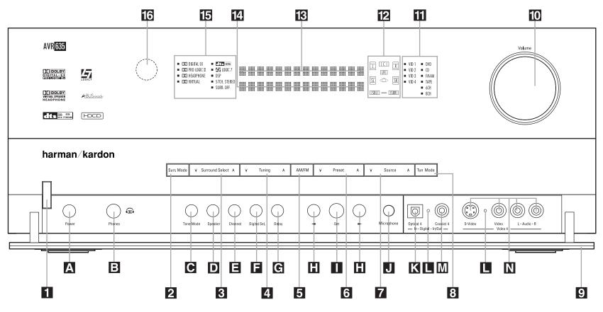
The following controls and indicators are available on the AVR 635's front panel:
